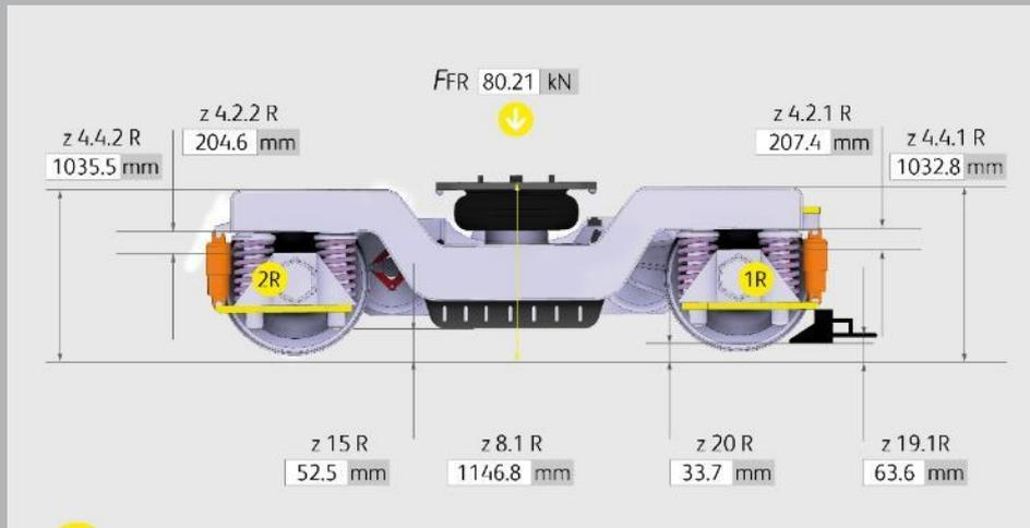
Checking heights under simulated load
