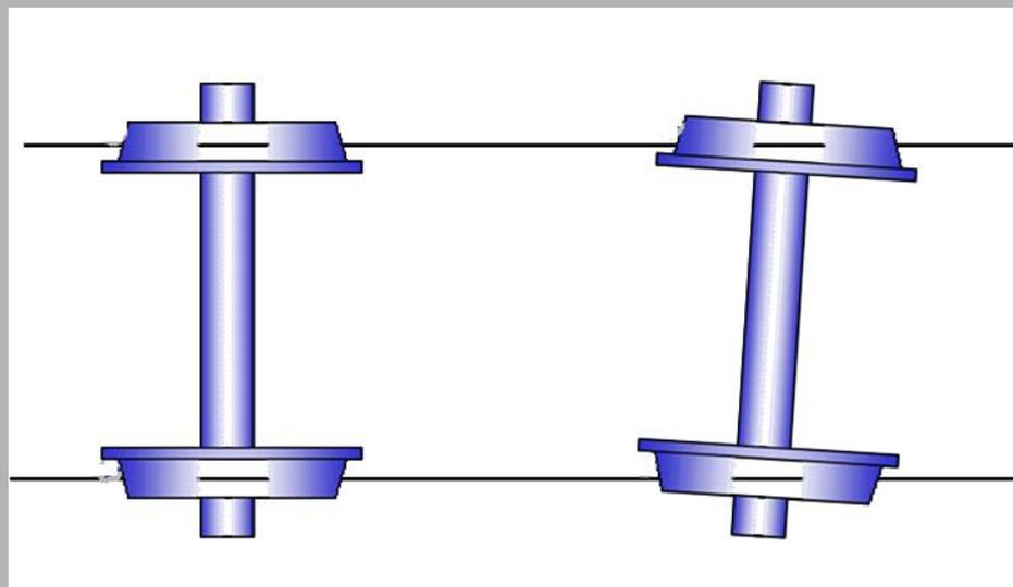
Un-parallel axles cause wearing and reduce the safety
