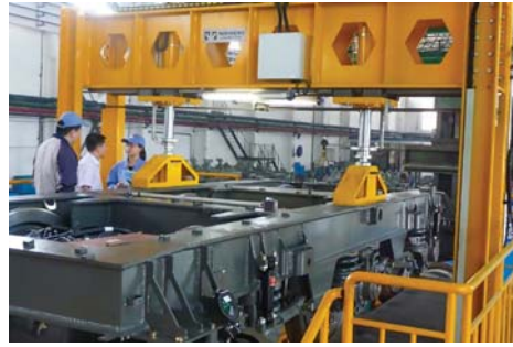
Checking the load distribution and other adjustments on the bogie test stand
