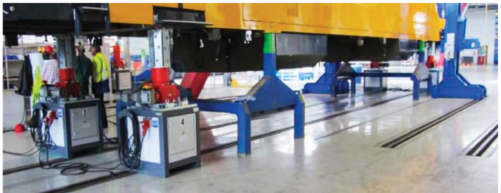
Determination of the load which the vehicle body applies onto the bogie RB
