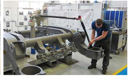
Checking the load distribution and other adjustments on the bogie test stand
